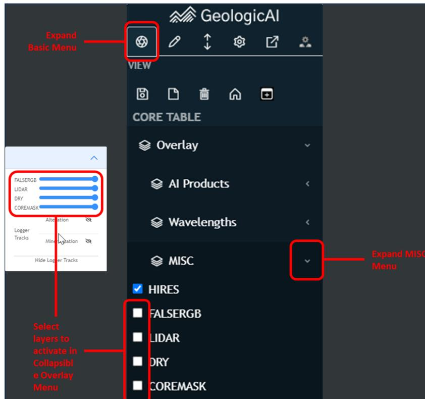
Figure 10: How to activate MISC features in Core Table.
