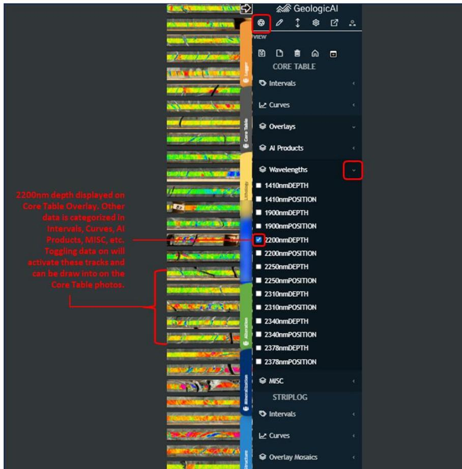
Figure 12: Toggling Tracks on Core Table Overlay.
