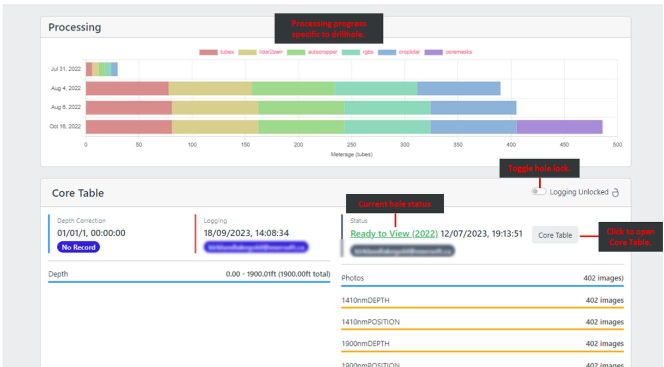
Figure 3: Drillhole specific submenu with processing statistics, drillhole locking, and Core Table access.
