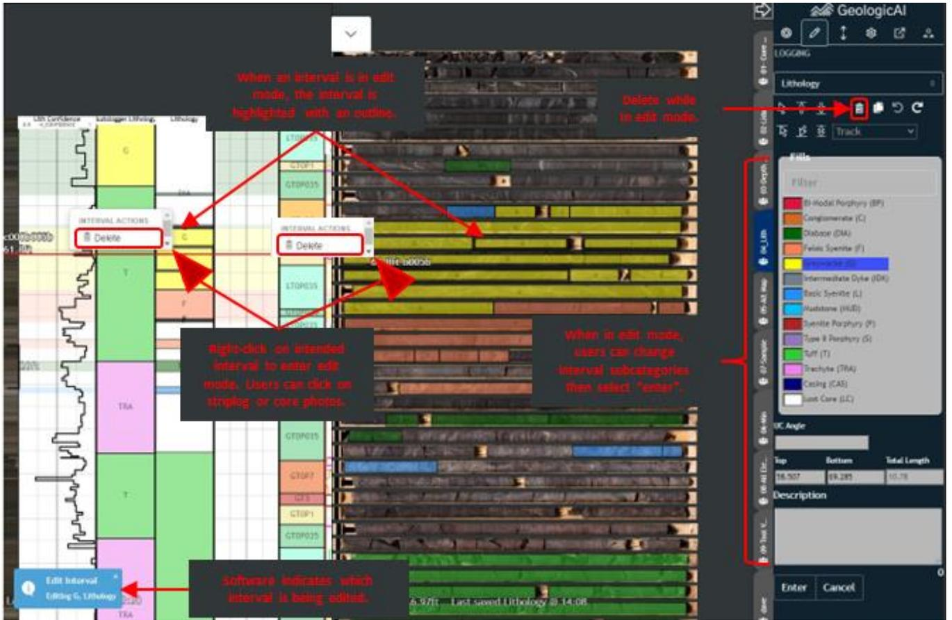
Figure 14: Steps to edit or delete an existing interval in Core Table.
