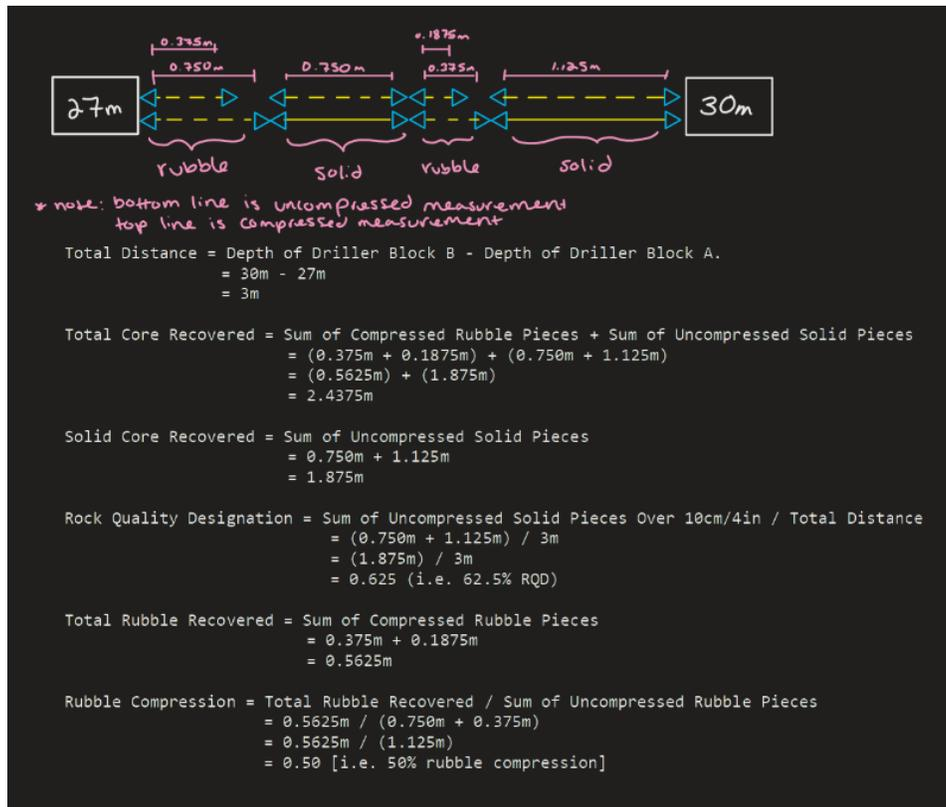
Figure 19: Backend calculations pertaining to RQD export values. This figure displays how calculations are conducted based on line types, compression, and expansion values. Note: Auto-Depth & Force-Depth will affect is compression and expansion (Table 4: Reference List for Figure 17).
