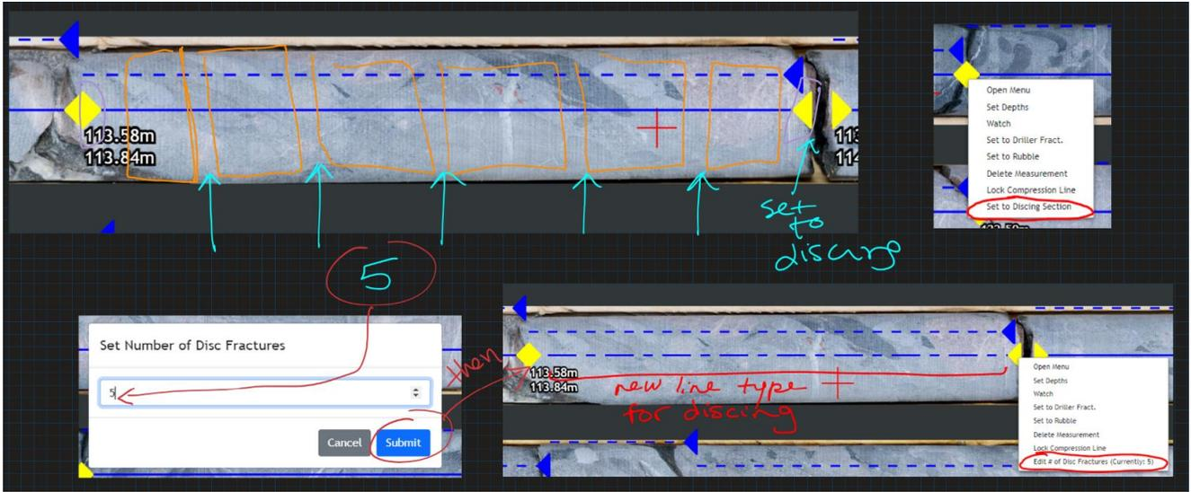
Figure 20: Recording discing parameters in Core Table.
