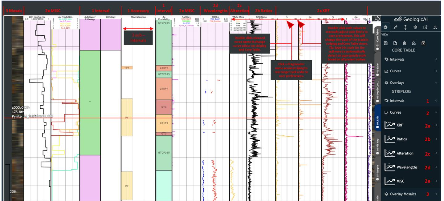
Figure 13: Striplog window and basic functionalities and types of tracks in Core Table.
