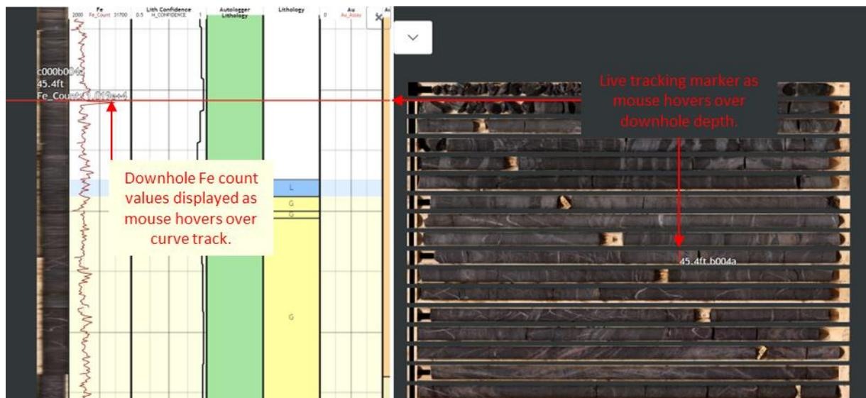
Figure 5: Live mouse tracking with downhole depths in striplogs and core photos.
